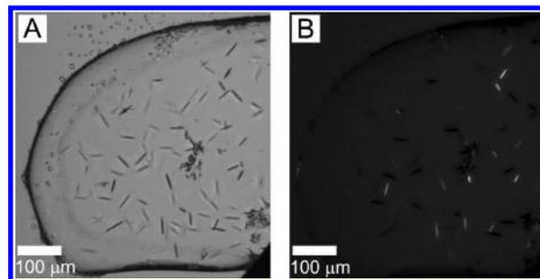
**Figure 7.** OprB crystals growing in the cubic mesophase formed by 8.7 MAG. Precipitant conditions include 20% (v/v) triethylene glycol, 0.08 M ammonium sulfate, and 0.15 M glycine. Crystals appeared on day 3 and reached maximum size of 50 μm on day 7. Images recorded with normal and with polarized light are shown in panels A and B, respectively. Other conditions are as described in Section 2.2.3 and in the legend to Figure 4.
