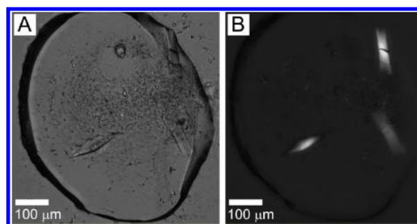
**Figure 8.** OprB crystals growing in the cubic mesophase formed by 6.9 MAG. Precipitant conditions include 21% (v/v) triethylene glycol, 0.05 M ammonium sulfate, and 0.15 M glycine. Crystals appeared after 16 h and grew to a maximum size of 40 μm × 100 μm in 7 days. Images recorded with normal and with polarized light are shown in panels A and B, respectively. Other conditions are as described in Section 2.2.3 and in the legend to Figure 4.
